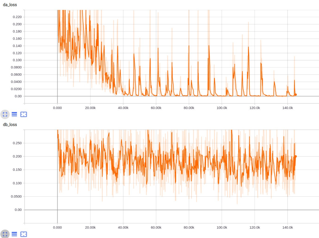
Fig. 4.9: Graphs showing Discriminator loss (on top: Lumidigm, on bottom: Secugen) with course of training. On Y-axis: Discriminator loss value, on X-axis: no. of steps in training
